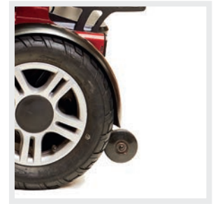
Anti-tilt wheels for stability and safety
